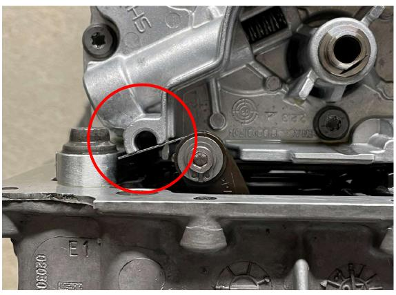
**2.** Fit the front cover back on replacing one torx bolt with the tensioner pin as pictured below. Put Loctite 270 on all fastener and pin threads, torque to 8nm.
