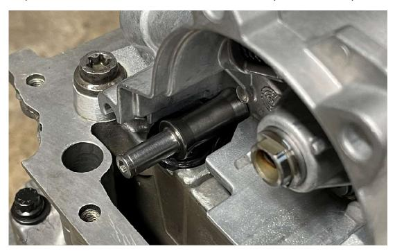
**3.** Fit the tensioner arm, spring, thrust washer and circlip as pictured below. Fit your oil pump chain and gear. Torque your new oil pump gear bolt to 5nm +90°.
